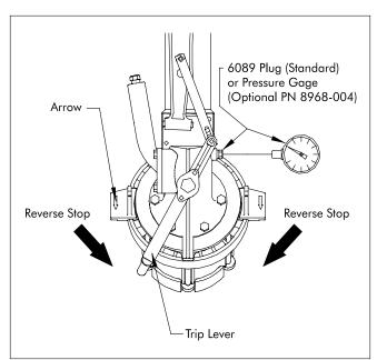
**3.** Adjust location of Reverse Stops to give desired arc of coverage. Stops must be mounted such that the arrows point towards each other with the Trip Lever located between them. If the Stops are set incorrectly on the wrong end of the arc, the sprinkler will fail to reverse.
