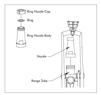
2. Install Nozzle on end of Range Tube. If using a Ring Nozzle, Install desired Ring size in Cap. Assure Ring is centered. Ring Nozzle Cap and Nozzle can be sufficiently tightened by hand.
