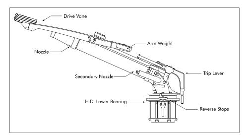
**NOTE ON LUBRICATION:** The SR200 sprinkler is lifetime lubricated and does not require periodic lubrication. The ball bearings in the H.D. lower bearing operate in a water resistant lubricant that is packed in the housing cavities and retained by seals. If repair of the lower bearing is done, it is recommended to use Nelson #6143 lubricant or a good grade of water resistant lubricant such as Lubriplate 130-AA.
