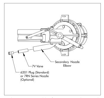
5. The SR200 is capable of using a Secondary Nozzle for in-close coverage. To use this feature, remove the supplied 6201 Plug and replace with the 7RN Series Nozzle of your choice. The supplied 7V Vane must be used to maintain proper stream integrity.
