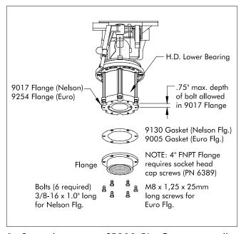
1. Securely connect SR200 Big Gun to traveller or riser designed to handle the loads of the operating sprinkler. Take care not to bottom out the bolts in the flange yet allow for at least 1/2" engagement of the bolt threads.
