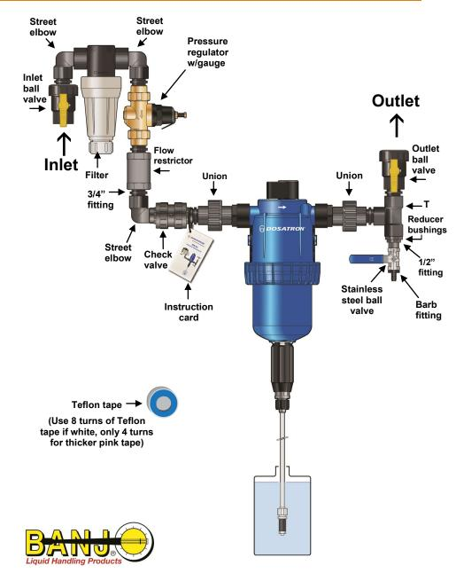
When connecting a DOSATRON either to the public water supply or to its own water source, you must respect the regulations in force concerning protection of the source i.e. backflow prevention, etc.
